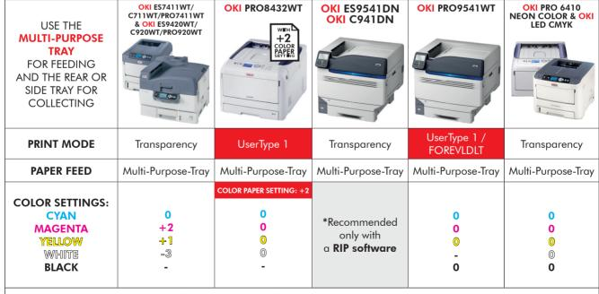
\*ATTENTION! When using a RIP software, the printer must be in factory settings.
